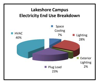
The plug load and lighting loads are significant, accounting for 23% and 28% of total electricity consumption. Approximately 40% of the plug load is attributed to the student residence. Reasons for this include the kitchen appliances found in each suite, including a large fridge and
