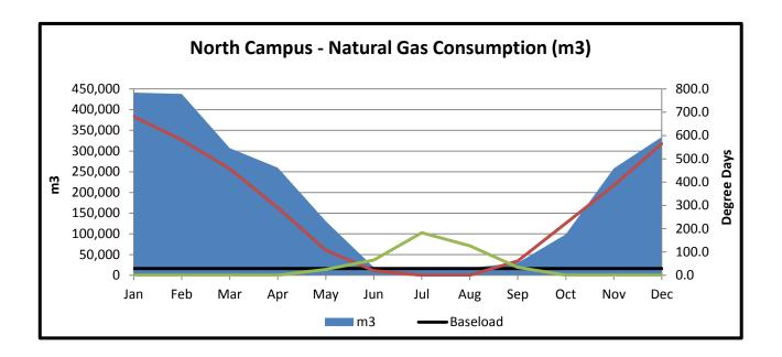
The natural gas profile coincides with the heating load. This is expected as natural gas boilers and rooftop units are the source for space heating. The small baseload during the summer months is attributed to natural gas domestic hot water heaters.
