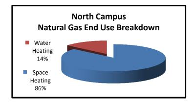
Space heating uses the majority of the total natural gas consumption, at 86%. This large space heating load is typical in climates such as Toronto's.
