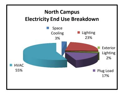
The mechanical systems load is significant, accounting for 55% of the total electricity load. Many of the ventilation and pump systems are over 45 years old, which could be one of the contributing factors to this end use. The plug and lighting loads account for 40% of the electricity. As mentioned, these end uses contribute to the baseload. By targeting these in the energy conservation measures, electricity decreases across the calendar year may be realized.
