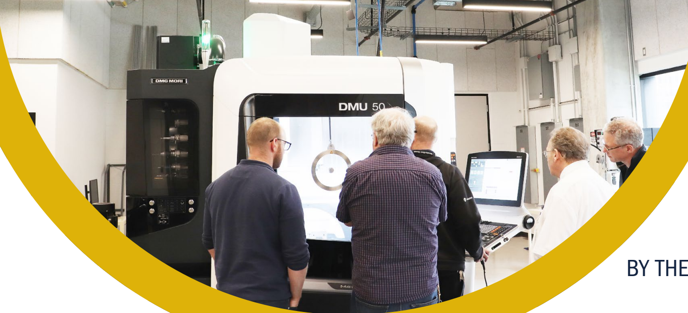
◀ DMU 50, 5-axis simultaneous CNC Machining Centre located within the Product Prototyping Facility in the Barrett CTI.
