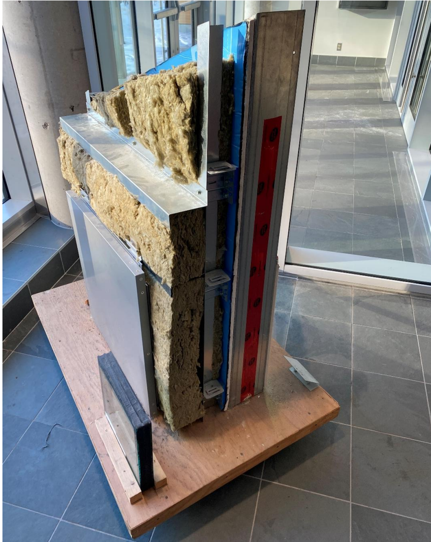
Figure 2: Example of Building Envelope Construction Mock-Up
